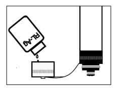
6 Screw the safety cap with the probe on the screw cap.
