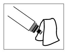
3 Screw the cleaning cap on the probe instead of the membrane head.
