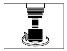
3 Thoroughly rinse the probe head with deionized water.
