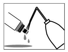
6 Immerse the probe head and the electrode unit into deionized water.
