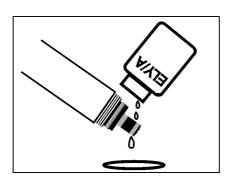
9 Screw the WP 25 membrane head on the shaft. Hold the probe inclined. Excess electrolyte solution is pressed out at the vent.
