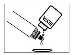
5 Screw the WP 25 membrane head on the shaft. Hold the probe inclined. Excess electrolyte solution is pressed out at the vent.
