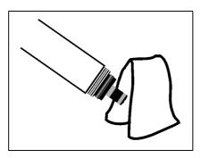
Moisten the new membrane with some drops of the ELY/A electrolyte solution.
