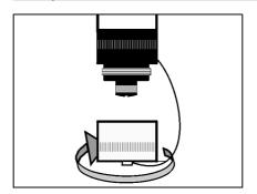
5 Fill the screw cap with RL-Ag/Oxi cleaning solution.
