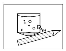
8 Rinse the probe head with electrolyte solution.
