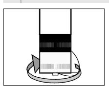
8 Thoroughly rinse the electrode - with the safety cap put on - with deionized water.-
