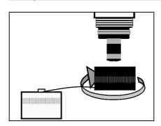
Thoroughly rinse the probe head and the electrode unit with deionized water several times.
