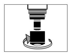
2 Using a lint-free paper towel, wipe the counter electrode and carefully remove any loose coating.
