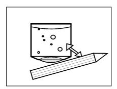
4 Rinse the probe head with electrolyte solution.
