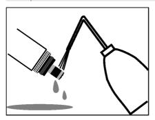
Soak the probe head and the electrode unit in deionized water for at least one hour.
