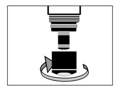
Thoroughly rinse the probe head with deionized water.
